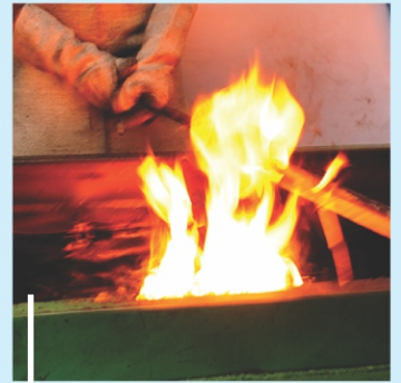
Oil Quenching of Gauges
